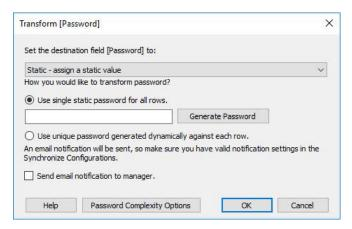
Figure 35: Transform dialog box for Password field
