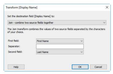
Figure 101: Transform dialog box -Join transform option
