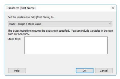
Figure 99: Transformation dialog box – Static transform option
