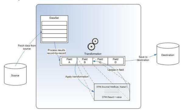
Figure 107: A high level representation of the mechanics involved in a transformation
